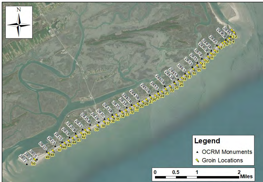
Figure 1. Overview of Folly Beach Groin Locations and Numbering. SCDHEC-OCRM Beach Survey Monument Stations also shown for reference.
